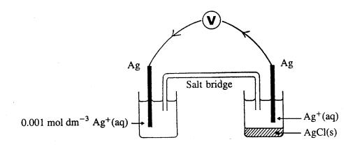
The potential of a silver ion/silver electrode is given by the Nernst equation
